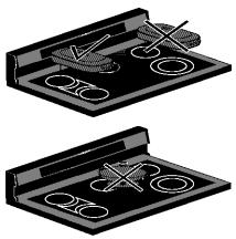
DO NOT use a wok if it is equipped with a metal ring. Because this ring traps heat, the cooktop surface could be damaged.
